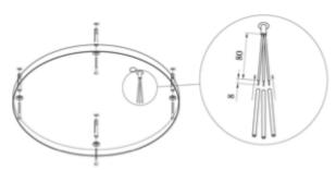
4. Extend the input cable through opening in the fixture and fix it to the wall/ceiling by using screws.
