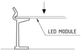
8.\*\* Mount the cable cover back to the fixture. 9.\* Insert LED module back into the brackets in the original position and snap into the brackets.
