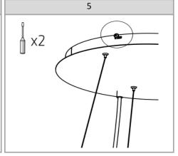
The product is intended for mounting on smooth and even surfaces. Permissible deviation of the ceiling surface from the plane marked on the two metre reference patch should not exceed 3mm. In case of larger ceiling deviations, it is necessary to consult the manufacturer as it is possible to purchase accessories for mounting on uneven surfaces.
